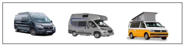
A base vehicle (van) is converted it into a panel van conversion usually marketed as a 'campervan' whereby the general structure of the van is kept and additional windows, high roofs or elevating roofs (pop-tops) are added.
